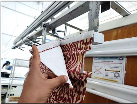
Picture 5. Valance with Velcro hook mounted on top of fabric material
