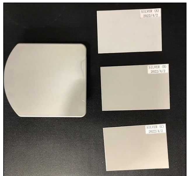
Picture 17. Paint chip samples “A”, “B” and “C” comparison against cassette 100 silver headrail end cap.
