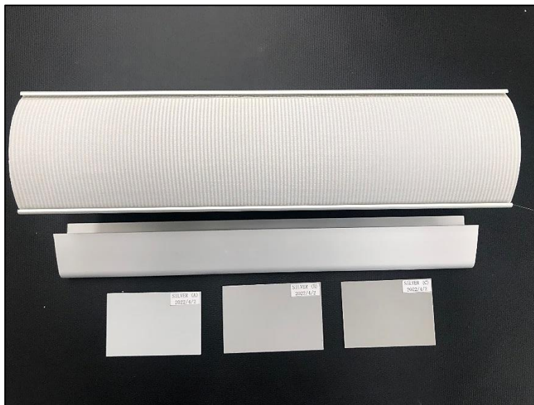
Picture 14. Silver V-Shaped bottom rail, Silver Cassette 100 headrail and paint color chip samples comparison.
