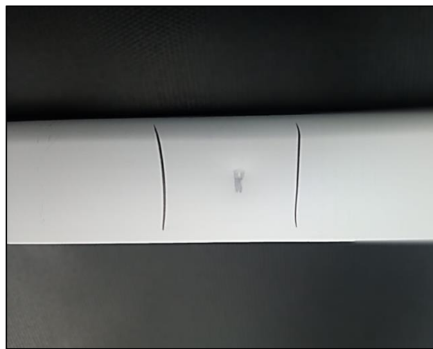
Picture 2. "Dents" or "Marks" damage by handling.
