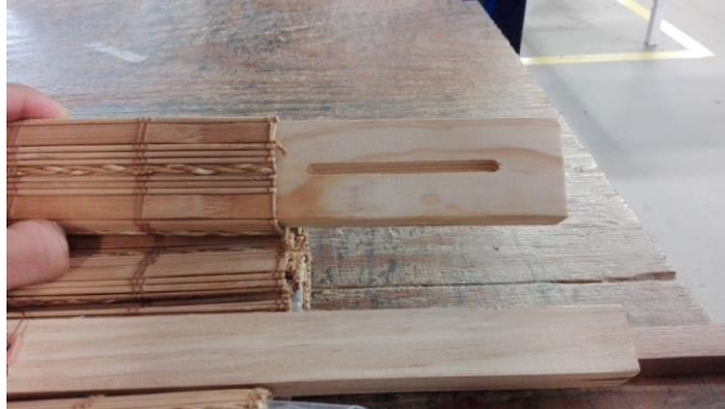
Figure. 3 Reveal after cutting the fabric trim on each side.
